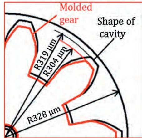
Fig. 15. Shrinkage of micro gear.
