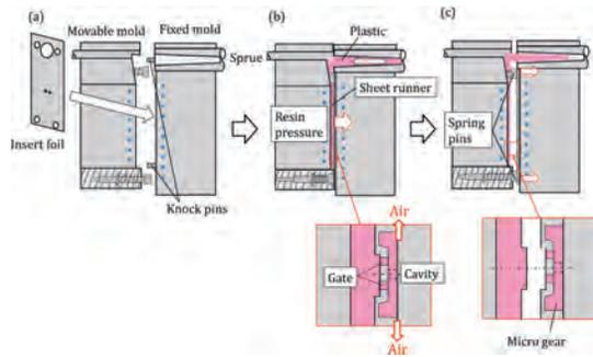
Fig. 6. Micro injection molding process.
