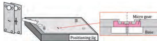
Fig. 9. Positioning on EDM machine.
