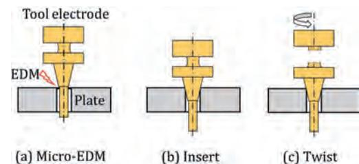
Fig. 1. Fabrication process of pin plate module.
