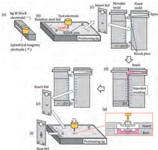
Fig. 3. Flow chart of EDM micro production system.
