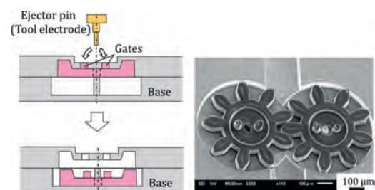
Fig. 10. Assembly of micro gears.
