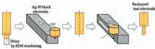
Fig. 11. Reshaping of rod.
