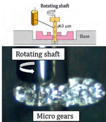
Fig. 13. Rotation of driving gear using rotation axis of EDM machine.
