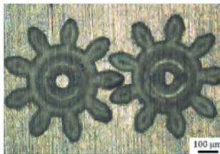
Fig. 7. Cavity of micro gears filled with plastic after injection molding.
