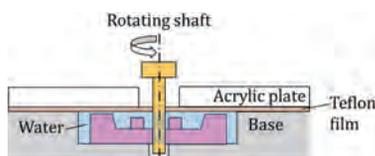
Fig. 14. Micro gear pump.
