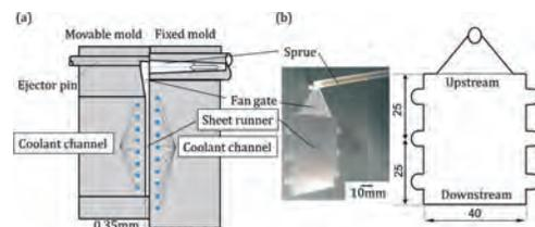
Fig. 5. Mold and molded plastic plate.
