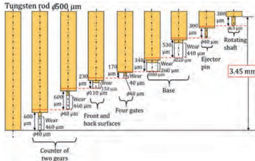
Fig. 12. Wear and removal length of rod.
